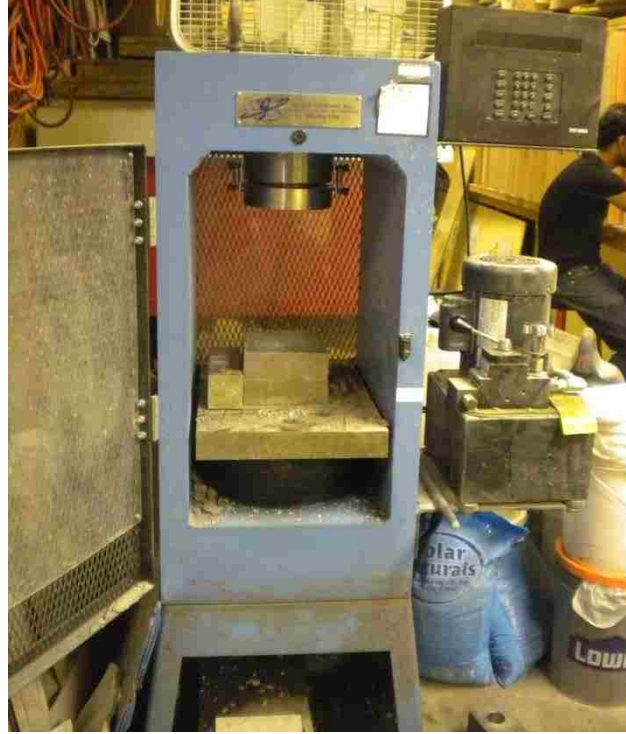
Figure 2.5: Compressive testing machine
