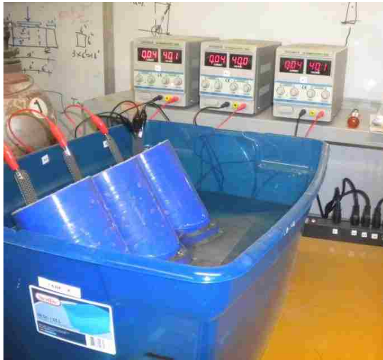
Figure 2.8: Rapid migration testing apparatus
