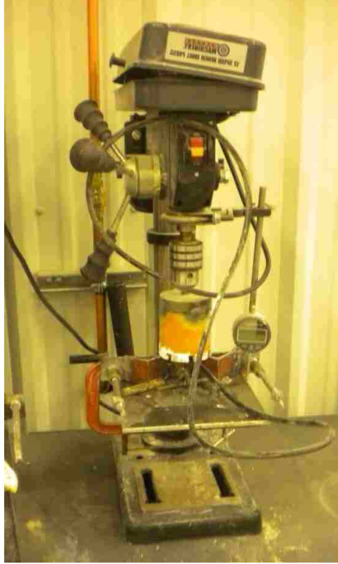
Figure 2.9: Power grinder for chloride diffusion test
