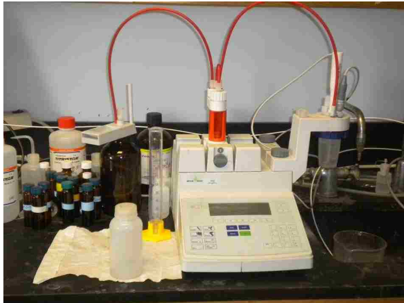
Figure 2.10: Automatic titration device for chloride diffusion
