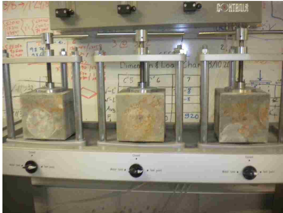
Figure 2.6: Water penetration testing apparatus
