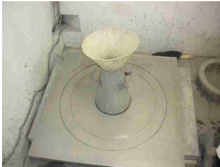
Figure 2.2: Slump flow test apparatus
